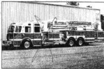
2007 E-ONE 95-foot mid-mount aerial – North Syracuse Fire Department, North Syracuse, N.Y.: E-ONE Cyclone II cab and chassis; Detroit Diesel Series 60 515-hp engine; Hale 2,000-gpm pump; 250-gallon tank; Harrison 10,000-watt hydraulic generator; Akron Brass 1,250-gpm monitor. $897,000. Dealer: Bob Liberatore, Absolute Emergency Vehicles & Equipment, Endicott, N.Y.
