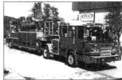
2008 Pierce tractor-drawn aerial – Tampa (Fla.) Fire Rescue: Pierce Quantum cab and chassis; Detroit Diesel Series 60 470-hp engine; Pierce TAK-4 independent front suspension; EMS compartment in cab; FireCom intercom system; 100-foot heavy-duty ladder; Harrison 10,000-watt hydraulic generator. $882,000. Dealer: John Thompson, Ten-8 Fire Equipment, Bradenton Fla. (Don Feipel Photo)
